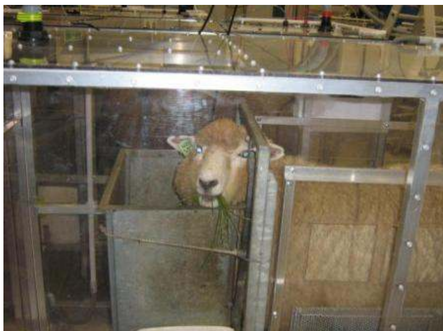
Figure 1.4 A sheep in respiratory chamber (photo courtesy of PGgRC)
