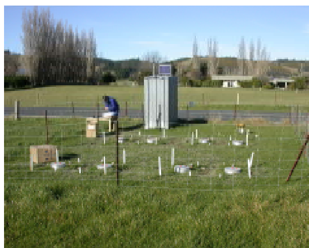
Figure 1.6 Measuring nitrous oxide emissions with collection chambers (photo courtesy of AgResearch).
